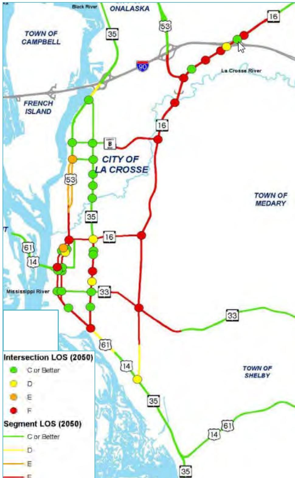
Figure 12: Future roadway capacity and level of service, 2050. Source: Coulee Region Transportation Study presentation materials.
