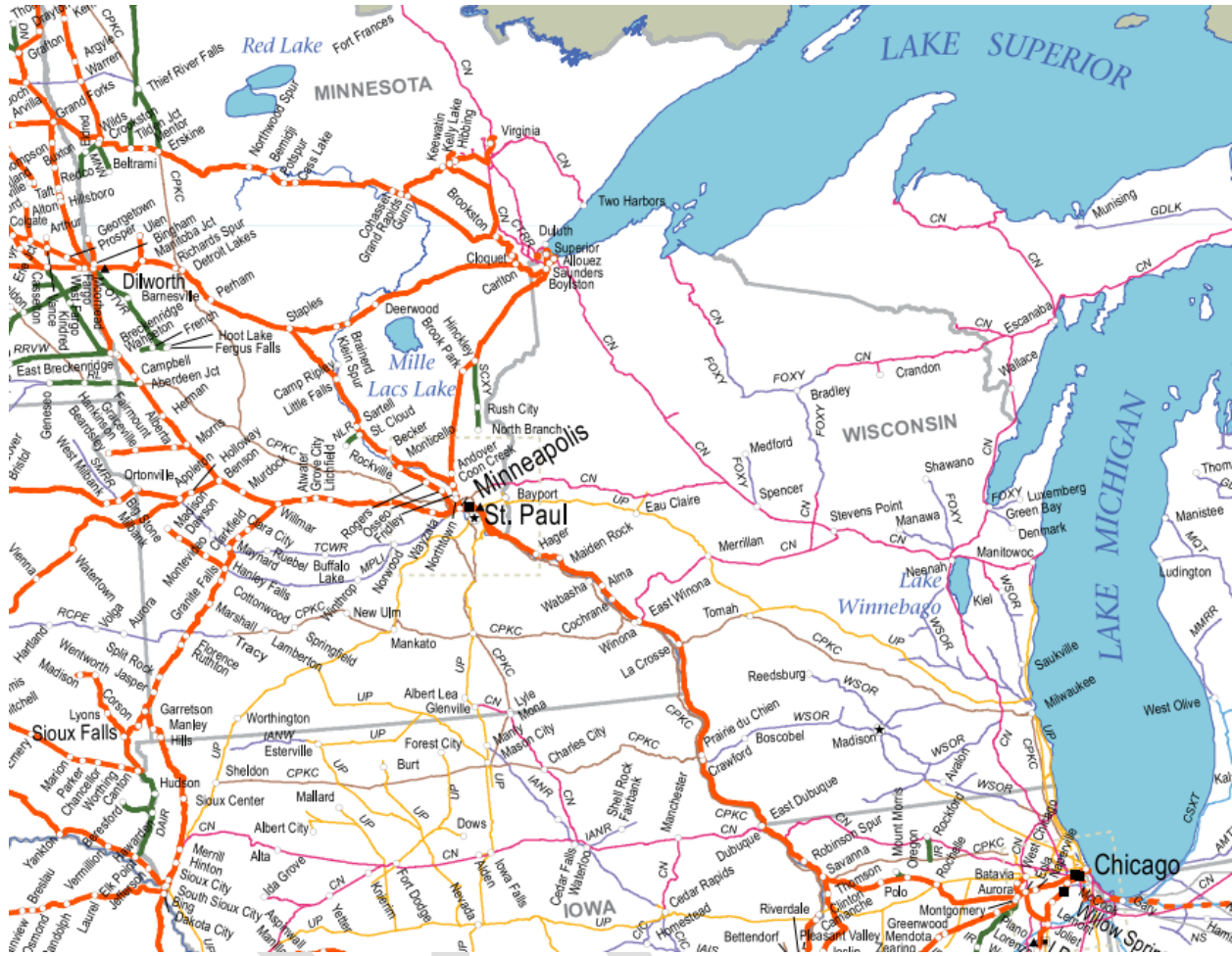
Figure 4.7. Snapshot from rail network map of Minnesota and Wisconsin region. The orange lines represent the Burlington Northern & Santa Fe network. Black circle symbols represent rail yards, black squares are intermodal facilities, and black triangles are automotive facilities. Other colored lines represent other rail networks. Source: www.bnsf.com . Created by Bartlett & West, May 2024.
